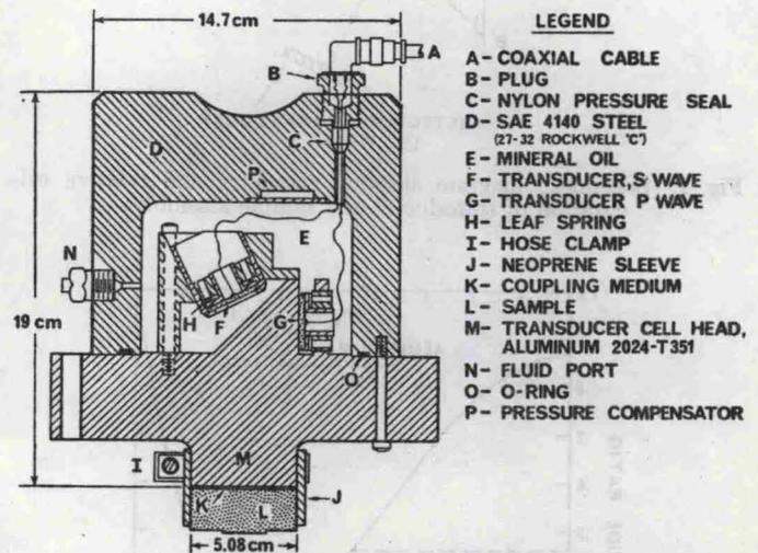
Fig. 5. Detailed cross section of transducer cell.
