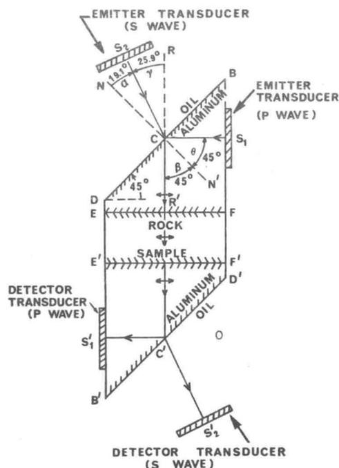
Fig. 1. Schematic diagram showing geometry and relative orientation of transducers and sample assembly.
